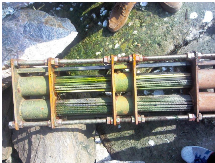
Figure: 3 Specimens of 8 mm RockRebar™ test sections appearance after removal from 6 months in iron cage and exposed to ocean splash zone shows only green moss.
