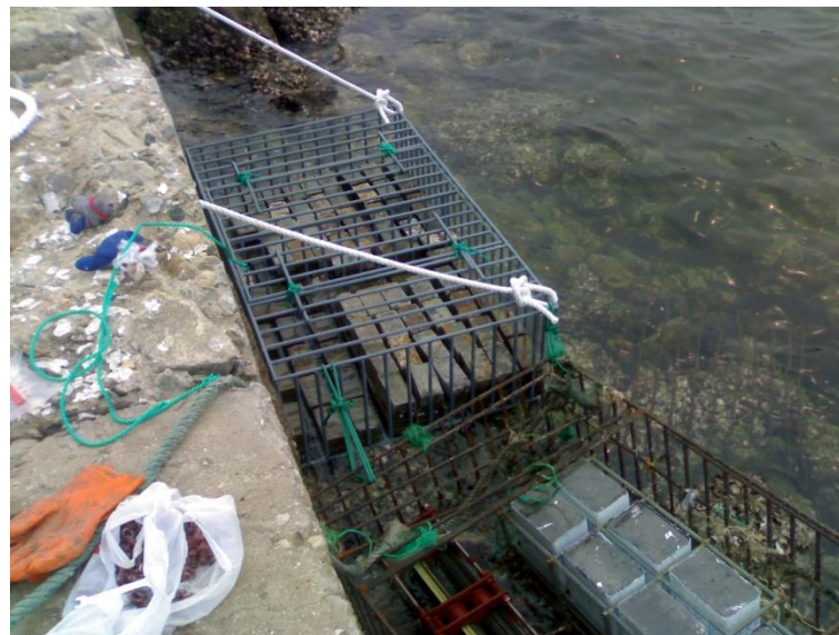
Figure 1: Sample: BFRP durability test in ocean splash zone.
