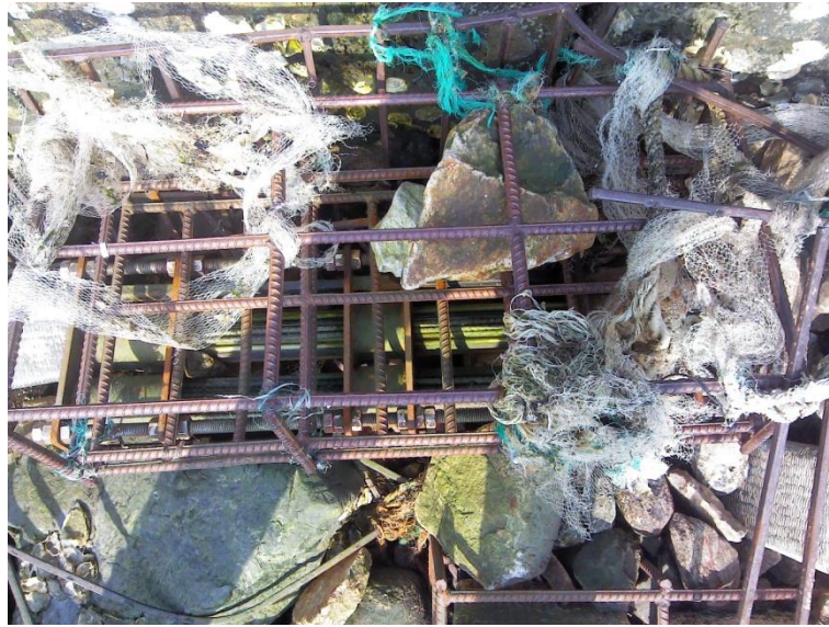
Figure: 2 shows appearance after 6 month and still inside the iron test cage (shown drying out at the ebb tide)
